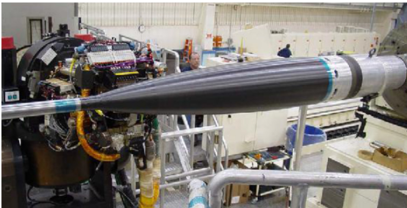
Fig. 2. Boeing Co. machine shown fabricating a composite laminate pressure hull by laying hoop fibers.
