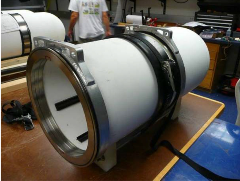
Fig. 1. Ceramic pressure hull of 11,000-m HROV "Nereus."
