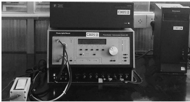
Fig. 1. The system for impedance spectroscopy measurement.
