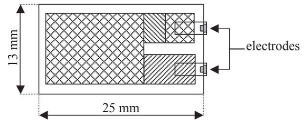
Fig. 2. Piezo film geometry characteristics.
