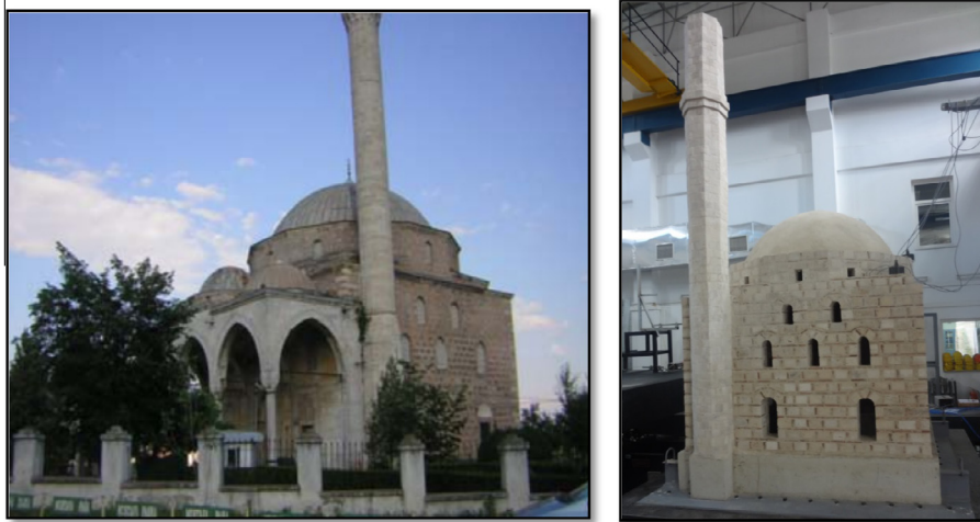
Fig. 1. Image of Mustafa Pasha Mosque in Skopje, Macedonia [17] on the left; 1:10 scale shake table model of the mosque on the right.
