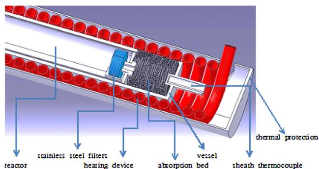
**Fig. 2.** Section view through the experimental reactor.
