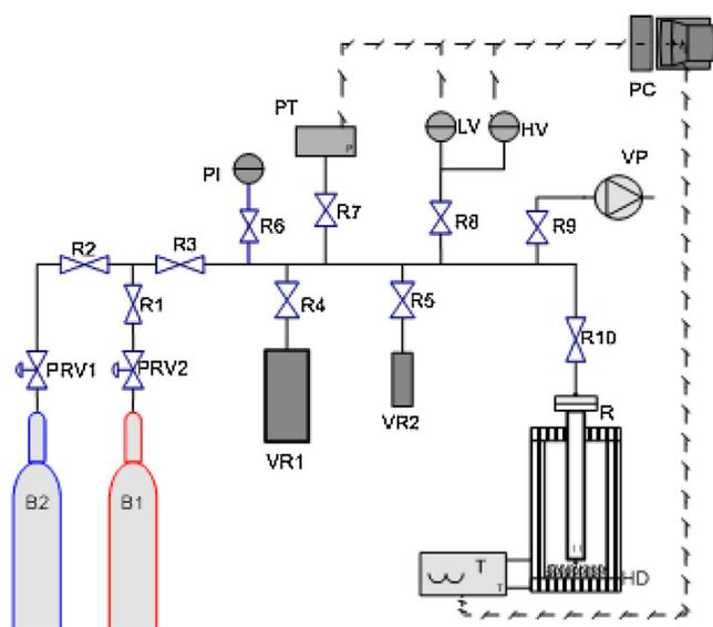
**Fig. 1.** Hydrogen isotopes storage & recovery experimental installation. Specific components: PRV1-2 – pressure reducing valves, R1-10 – automatically isolating valves, B1 – hydrogen tank, B2 – deuterium tank; VR1 – metering vessel 1, VR2 – metering vessel 2, LV – low vacuum gauge, HV – high vacuum gauge, PT – pressure transducer; PI – pressure indicator; VT – high vacuum train; R – reactor; HD – heating device.
