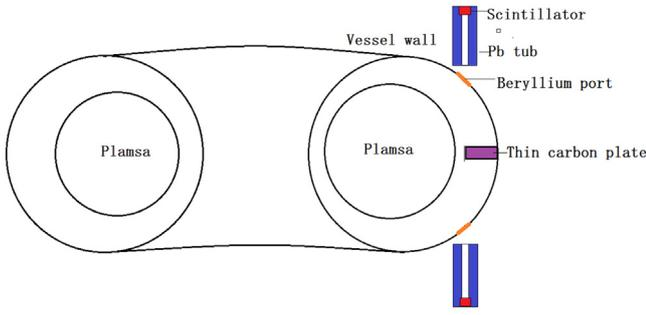
**Fig. 1.** Experimental design consisting of a thin carbon plate inserted at the plasma edge where plasma positron annihilation occurs, two beryllium ports to prevent the scattering of annihilation photons, and two scintillators with collimators to detect coincident annihilation photons.
