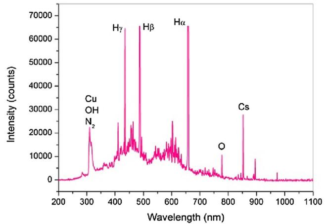
Fig. 3. The typical spectrum of the initial phase of source operation with H<sub>2</sub> gas and Cs injection, hydrogen atomic and molecular lines, Cs atomic lines along with some impurity lines are visible.
