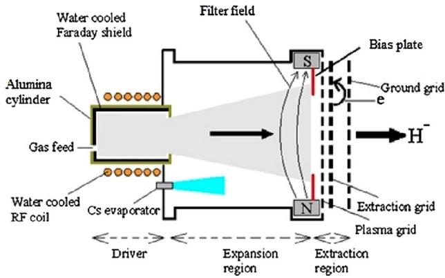
Fig. 1. Schematic of the negative ion source; ROBIN.
