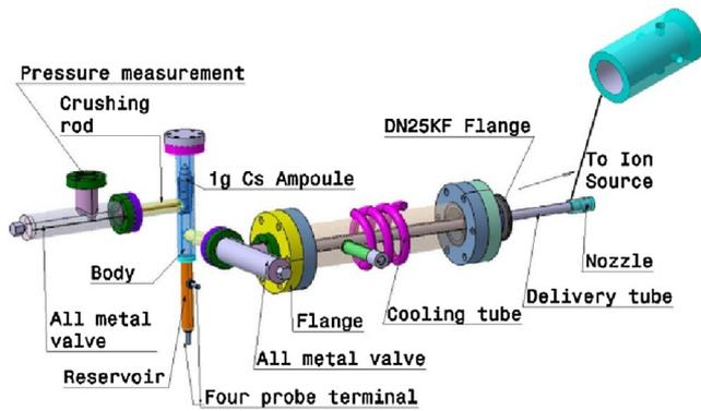
Fig. 2. Schematic of Cesium delivery system.
