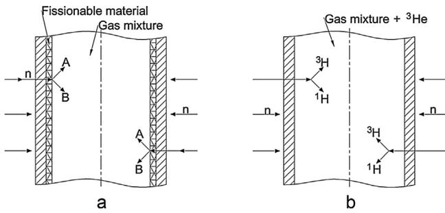
Fig. 1. Gaseous medium excitation methods: a – surface sources (Reactions (1)–(4)); b – volume sources (Reaction (5)).
