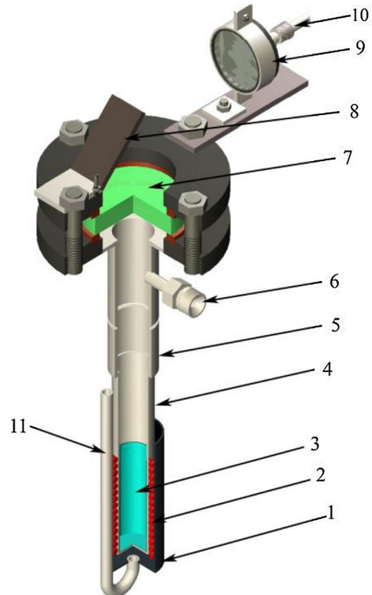
Fig. 3. Reactor AD for studies of optical radiation of nuclear-excited plasma: 1 – cooling casing; 2 – heater; 3 – (lithium) fissile materials thin layer; 4 – experimental cell body; 5 – AD body; 6 – gas mixture pumping and supply tract; 7 – quartz window; 8 – hinged mirror; 9 – collimator; 10 – fiber-optic lightguide; 11 – cooling tract.
