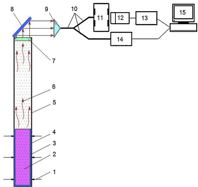
Fig. 2. Scheme of experiments on study of optical radiation of nuclear-excited plasma: 1 – thermal neutron flux; 2 – gas mixture excited by <sup>6</sup>Li(n,α)<sup>3</sup>H reaction's products; 3 – Li layer; 4 – experimental cell; 5 – housing of ampoule device; 6 – optical radiation; 7 – quartz window; 8 – hinged mirror; 9 – collimator; 10 – optical fiber; 11 – monochromator; 12 – photosensor; 13 – oscillograph; 14 – optical spectrometer; 15 – PC.
