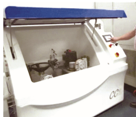
Fig. 2. Salt spray chamber used for Enduro™ product testing.
