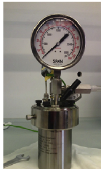
Fig. 1. Temperature controlled stainless steel autoclave.
