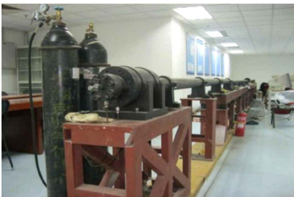
Fig. 2. The test device of SHPB.
