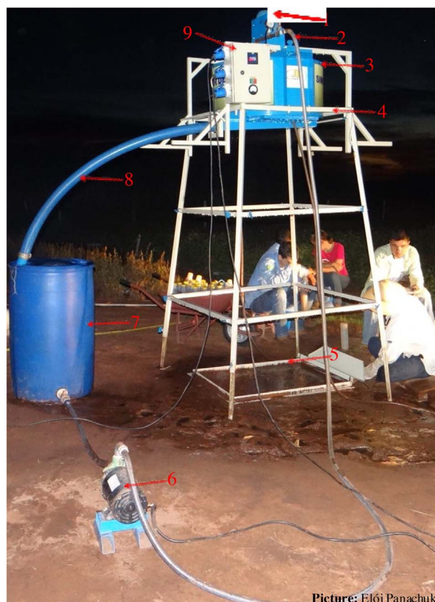
Fig. 1. The portable rainfall simulator InfiAsper during a rainfall application in bare soil system: 1 – motor, 2 – water application, 3 – blocking device, 4 – upper frame, 5 – runoff collector, 6 – water pump, 7 – tank, 8 – excess water collector and 9 – electric panel control.
