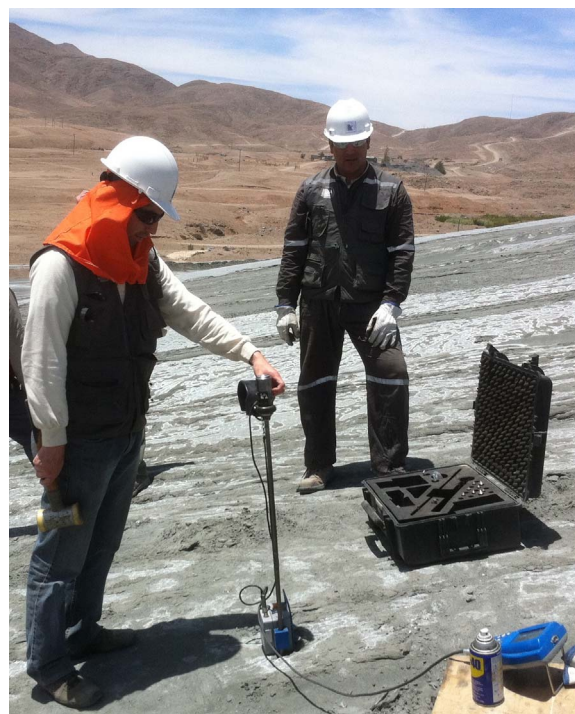
Fig. 2. PANDA 2 operation on soft soil. The operator (left) has the mallet in his hand. The logger (bottom right) displays calculated resistance in real time. All equipment fits into the carrying case for transport.
