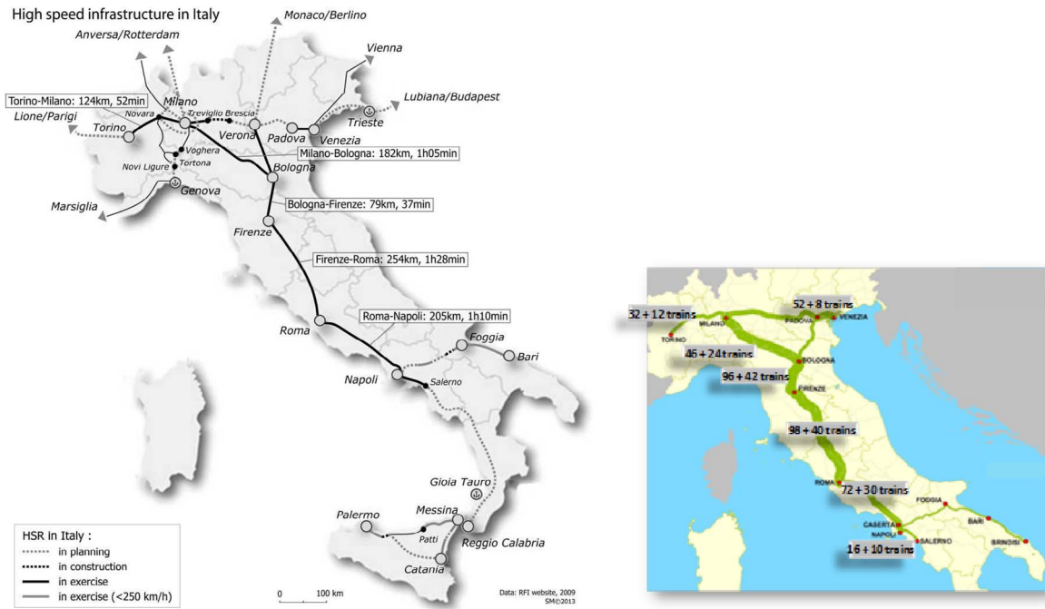
Fig. 1. The High-Speed/High-Capacity Rail system in Italy. (The total number of trains along each corridor is reported considering the two companies Trenitalia and NTV.)
