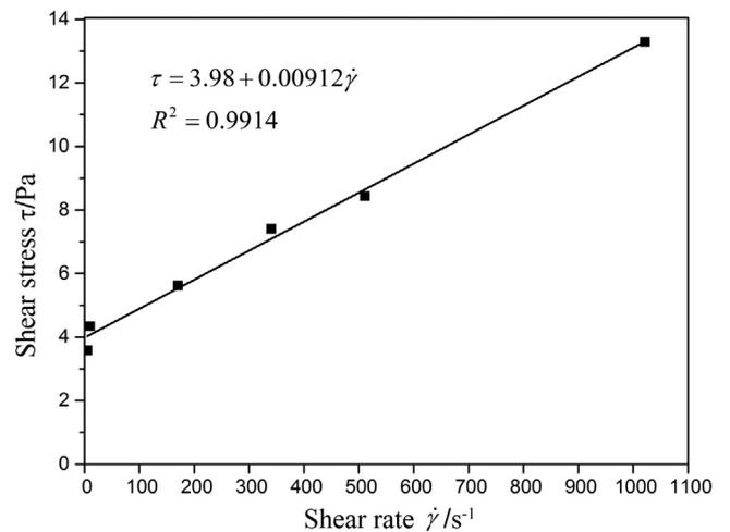
Fig. 1. The rheological curve of slurry.
