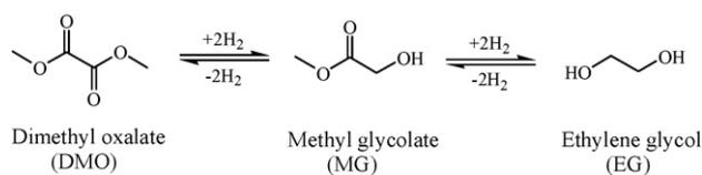
**Scheme 1.** The hydrogenation process of the DMO.
