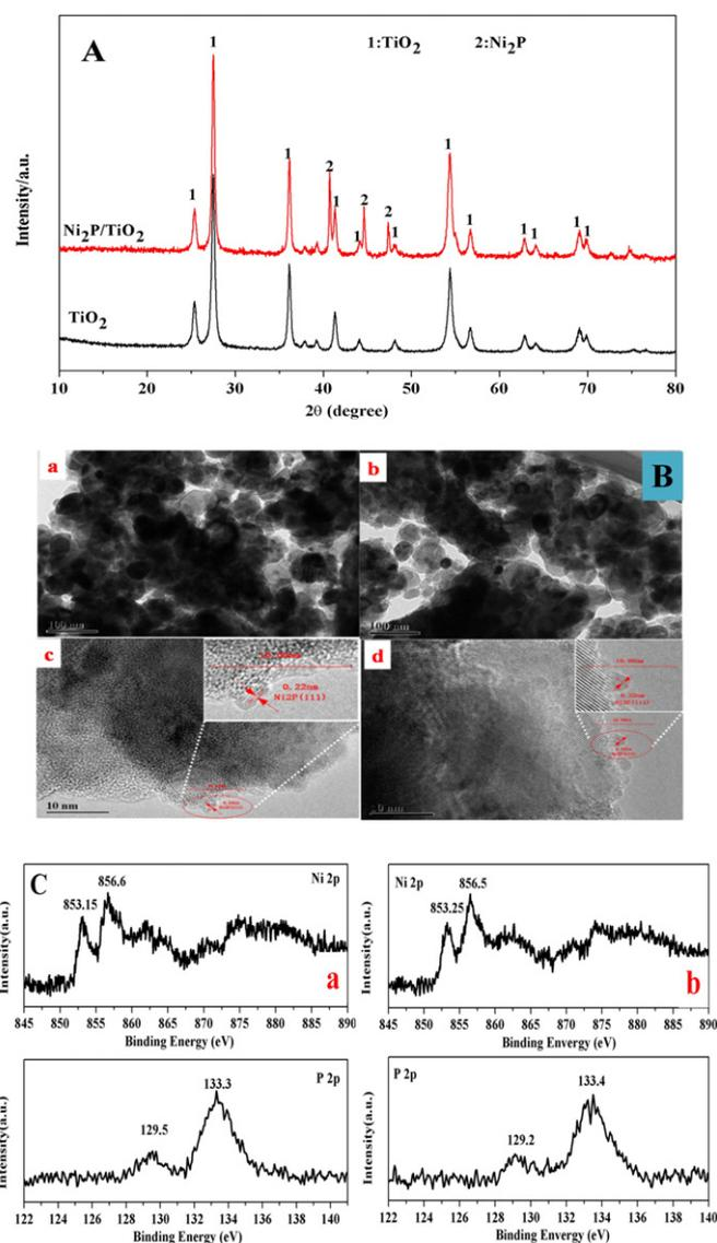
**Fig. 1.** (A) XRD patterns of as-prepared Ni<sub>2</sub>P/TiO<sub>2</sub> catalyst and TiO<sub>2</sub> support. (B) TEM and HRTEM images of the as-prepared (a and c) and spent (b and d) Ni<sub>2</sub>P/TiO<sub>2</sub> catalysts. (C) XPS spectra in the Ni (2p) and P (2p) regions for the as-prepared (a) and spent (b) Ni<sub>2</sub>P/TiO<sub>2</sub> catalysts.
