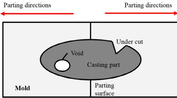
Fig. 1. Illustration of the two conditions under which the molds cannot be removed without damage.
