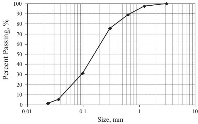
Fig. 1. Grain size distribution curve of sand.
