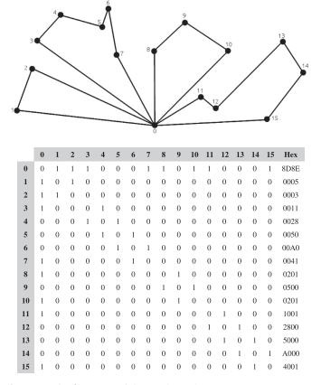
**Fig. 1.** Example of routes encoded as a spin matrix. Customer-customer connections are represented using single bits. The matrix is encoded row-wise to form hexadecimal (Hex) words which stored in memory as an array.
