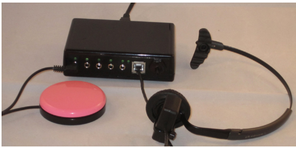
Fig. 1. The MultiPos system. From left to right: pink click device, communication part in a black box, head band with built-in MEMS gyroscope. (For interpretation of the references to color in this figure legend, the reader is referred to the web version of the article.)
