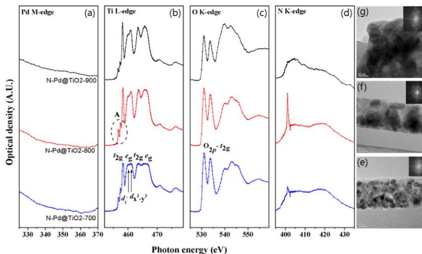
Fig. 2. XAS spectra of (a) Pd *M*-edge, (b) Ti *L*-edge, (c) O *K*-edge, and (d) N *K*-edge for N-Pd@TiO<sub>2</sub>-700 (blue line), 800 (red line), and 900 (black line), TEM images obtained from (e) N-Pd@TiO<sub>2</sub>-700, (f) 800, (g) 900.
