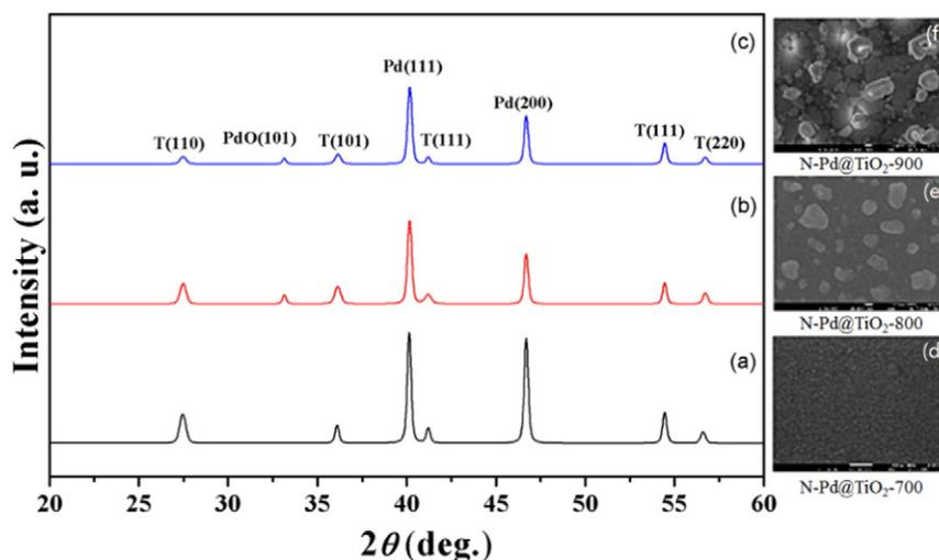
Fig. 1. XRD patterns and SEM images obtained from (a), (d) N-Pd@TiO<sub>2</sub>-700, (b), (e) N-Pd@TiO<sub>2</sub>-800, and (c), (f) N-Pd@TiO<sub>2</sub>-900.
