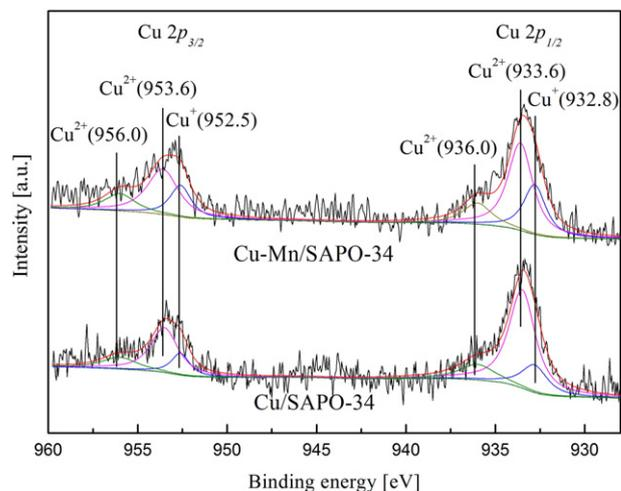
**Fig. 2.** Cu 2p XPS spectra of the catalysts.
