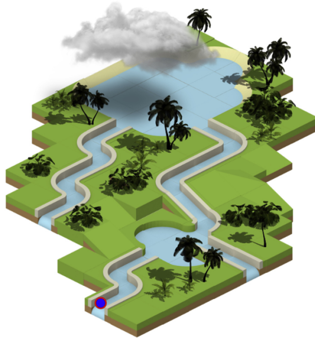
Fig. 1. An imaginary drainage network with flow limiting gate and/or water storage systems. The interesting signal is the level/flow at the outlet of the network, marked with a circle. Isometric tiles from www.kenney.nl .
