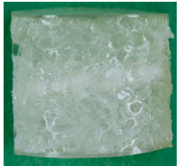
Fig. 2. Macroscopic image of the meniscal silk fibroin scaffold (FibroFix™, Orthox Ltd., Abindon, UK).
