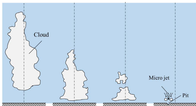
Fig. 1. Illustration of cloud collapse and pit formation.
