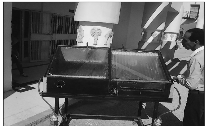
Fig. 1. Modified solar still (right) and conventional solar still (left).
