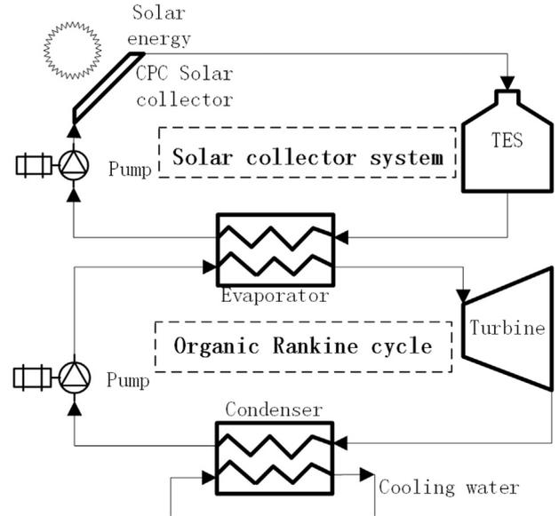
Fig. 2. Schematic diagram of the SORC power system.
