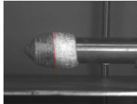
Fig. 2. Typical cavitation at  $t = 0.006$  s. The white foam like re-entry jet inside the cavity is marked by a red line. (For interpretation of the references to color in this figure legend, the reader is referred to the web version of this article.)
