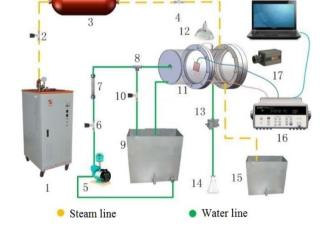
steam generator; 2, 4, 6, 10- trim valve; 3- superheater; 5- diaphragm pump; 7- rotor flow meter;
