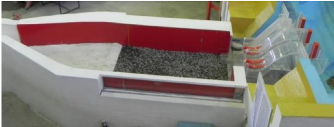
Fig. 2. 1:50 scale physical model of the Toachi ski jump (EPN, 2013).
