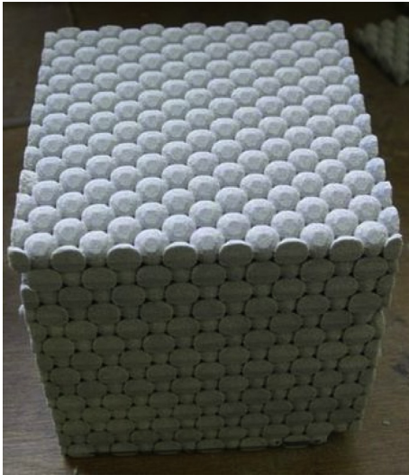
Fig. 2. The sand mould before infiltration by the liquid metal.
