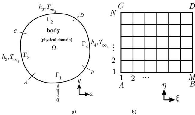
Fig. 1. Arbitrarily shaped two dimensional heat-conducting body (physical domain) subjected to convective heat transfer on surfaces  $\Gamma_i, i = 2, 3, 4$  and heat flux  $\dot{q}$  on surface  $\Gamma_1$  (a) and the corresponding computational domain (b). The thermal conductivity of the body is  $k_T$ .
