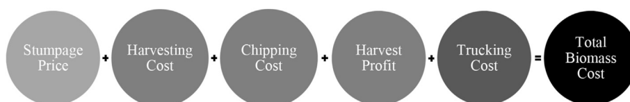
Fig. 1. Biomass Supply Chain Costs Cost of biomass delivered to purchasing facility (i.e., electricity generator, biorefinery).
