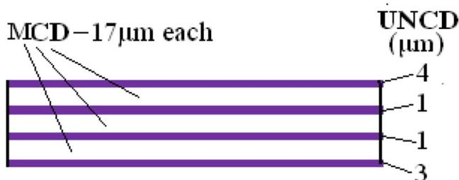
Fig. 1. A schematic diagram of the seven-layered-composite diamond with total thickness of 60  $\mu\text{m}$  designed for THz TWT windows.
