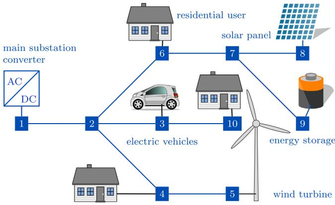
Fig. 1. Example of an LVDC system for urban area applications.
