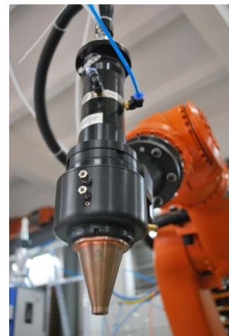
Fig. 4. A product of cladding head of HLB-IPF technology with series number of JGRF-102-2.
