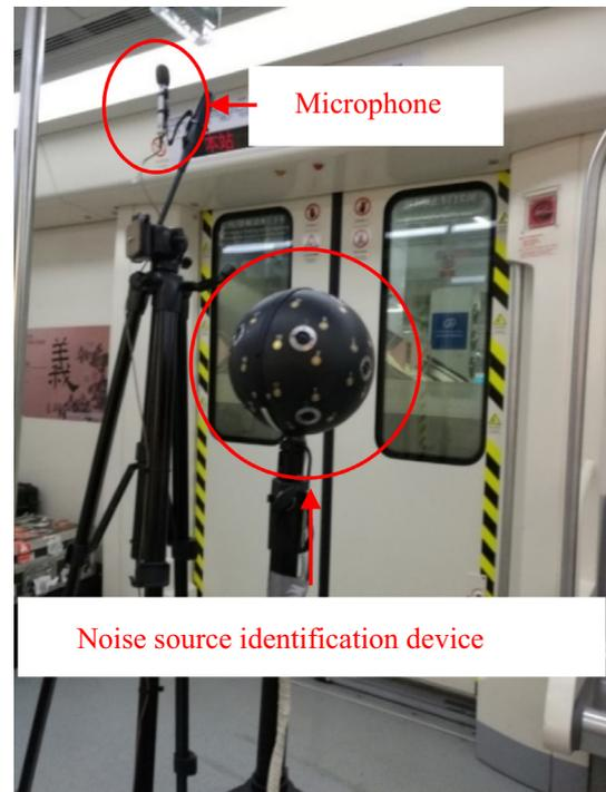
Fig. 1. Measurement points of interior noise and sound source identification.
