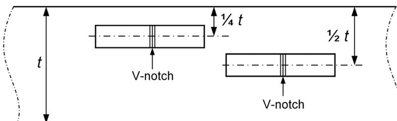
Fig. 2. Positions of thermal simulation specimens.
