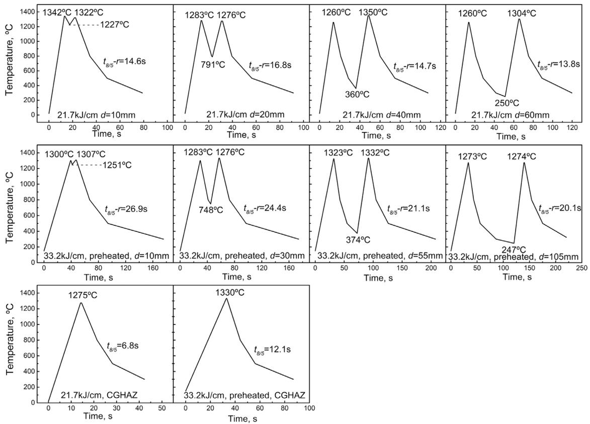
Fig. 1. Thermal cycles used for thermal simulation tests.
