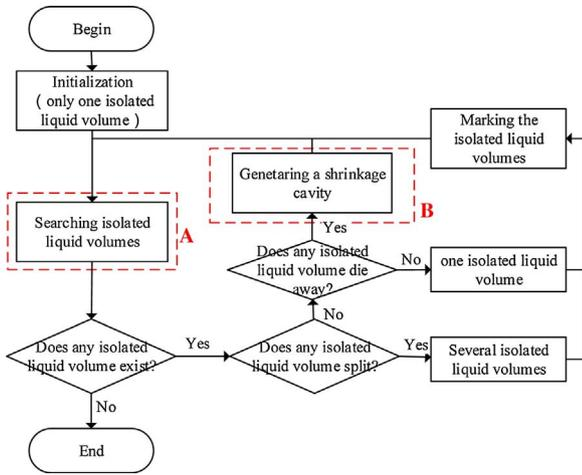
Fig. 1. Evolution of isolated liquid volumes in vertical centrifugal casting process.
