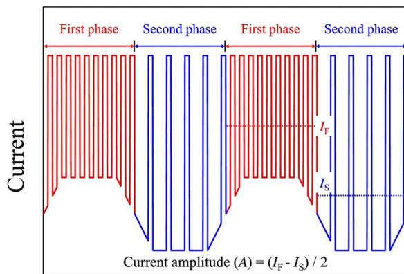
Fig. 1. Schematic diagram of current waveform of DP-GMAW. Current amplitude ( $A$ ) is defined as half of the difference between the average current of the first phase ( $I_F$ ) and the average current of the second phase ( $I_S$ ).
