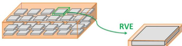
Fig. 1. The RVE of a sample with aligned graphene sheets.
