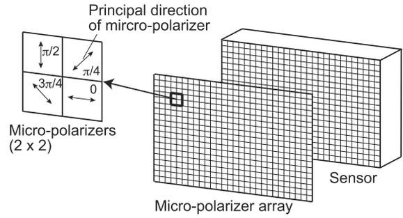
Fig. 1. Configuration of the micro-polarizer array on the sensor plane.
