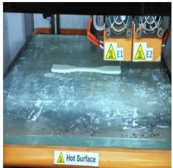
Fig. 3. FDM setup used for 3D printing.
