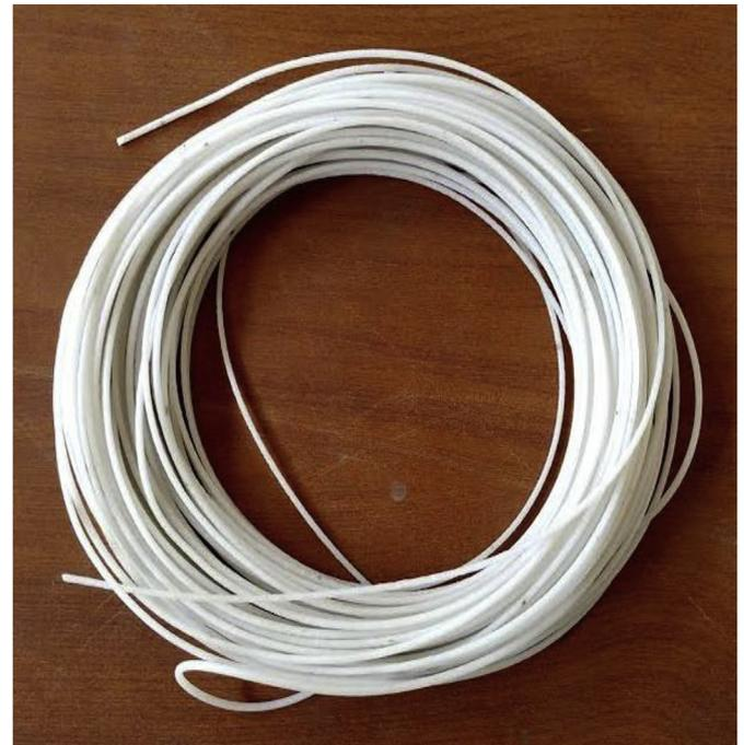
Fig. 2. In-house extruded FDM filament.
