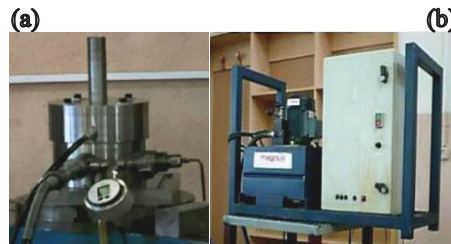
Fig. 2. (a) Hydrodynamic Deep Drawing assisted by Radial Pressure with Inward Flowing Liquid setup, and (b) hydraulic unit.
