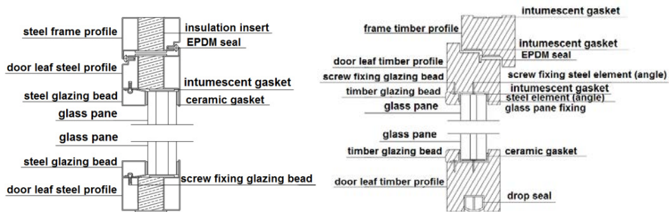
Fig. 1. Sample steel and timber profile cross-sections [8].
