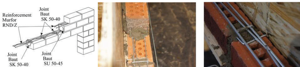
Fig. 2. A structural solution of brick lintels.
