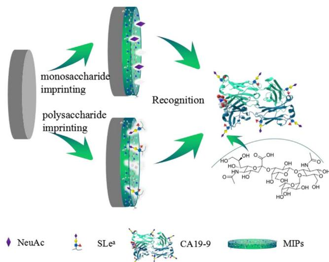
**Scheme 1.** Construction of a CA19-9 sensor based on glycosyl imprinting.
