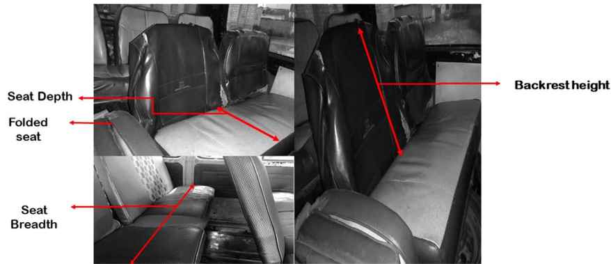
Fig. 1. Locally fabricated seats and interior view of the trotro vehicle.
