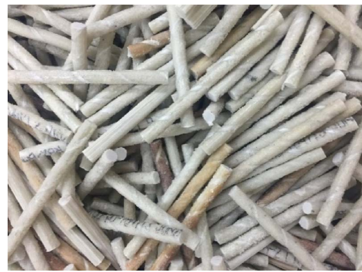
Fig. 2. FRP-Needles with a diameter of 6 mm and length of 100 mm.
