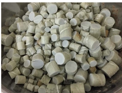
Fig. 1. FRP-RA used as a replacement of coarse aggregate in concrete.
