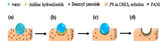
Fabrication of polystyrene honeycomb patterned porous films with polyaniline functionalized pores
